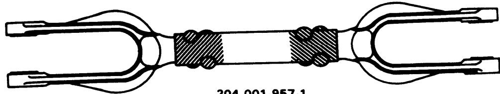
204-001-957-1 204-001-959-1 CONTROL TUBE ASSEMBLY
