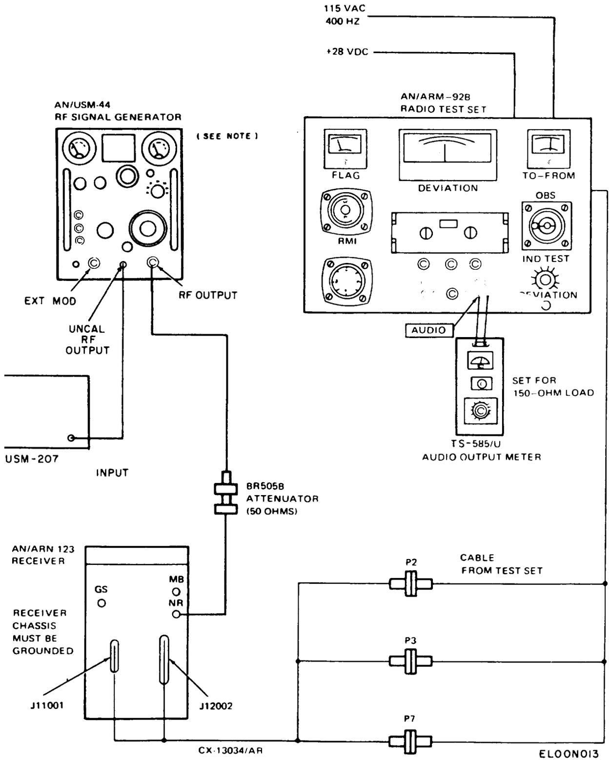
Figure 3-5. Bench Test Set, Alternate VOR/LOC Receiver Sensitivity Test.
