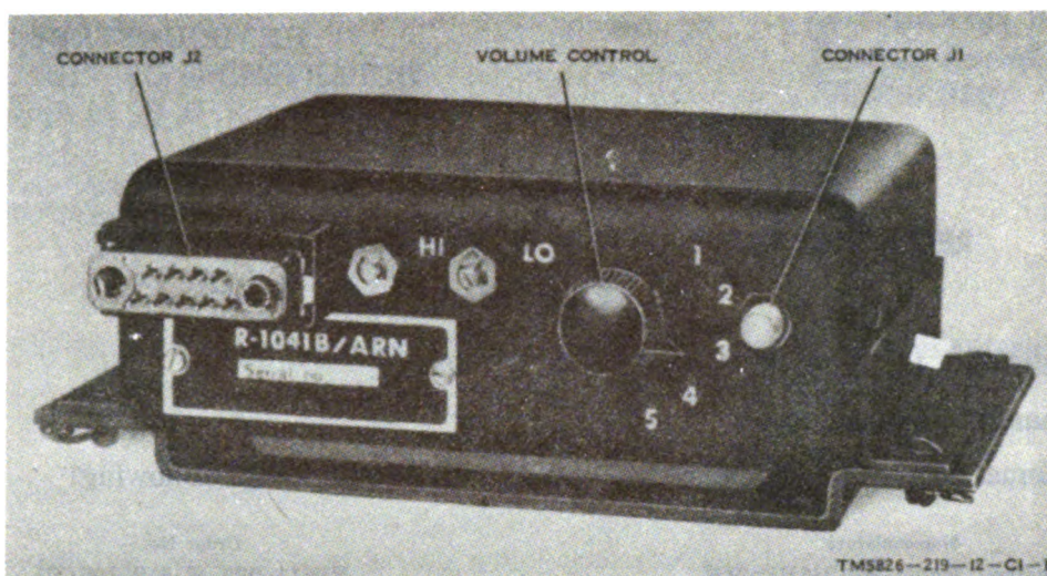
Figure 4. Receiver, Radio R-1041B/ARN attached to Mounting MT-2292/AR, rear view.
