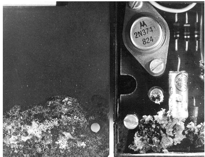
Figure 3-1. Corrosion Caused by Blown Capacitor Acid
