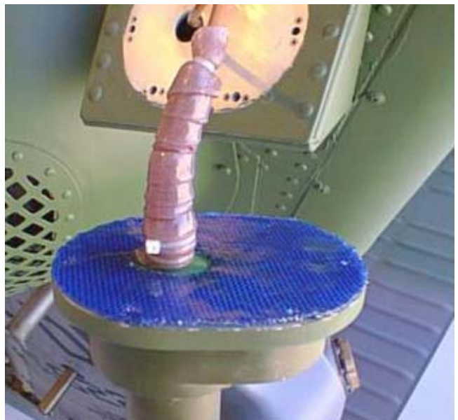
Figure 6-5. Stretch Seal Protective Wrap Applied to Antenna Connector
