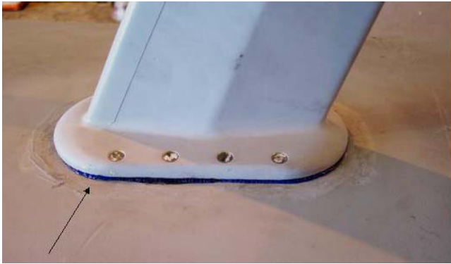
Figure 6-6. Typical Gel Squeeze-Out Around Perimeter of Antenna
