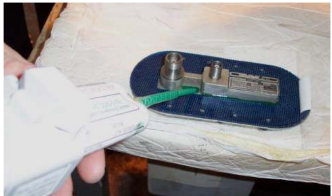
Figure 6-4. Application of Self-Leveling Green Sealant
