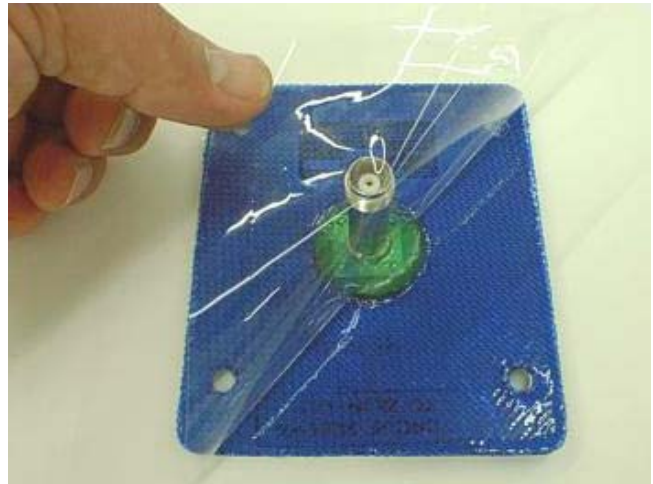
Figure 6-3. Removal of Release Film From Gasket
