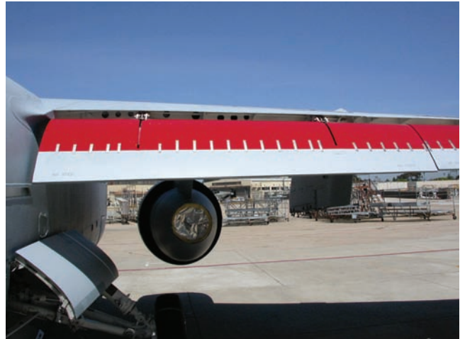
Figure 3-15. Flaps Lowered to Expose Recess Areas
