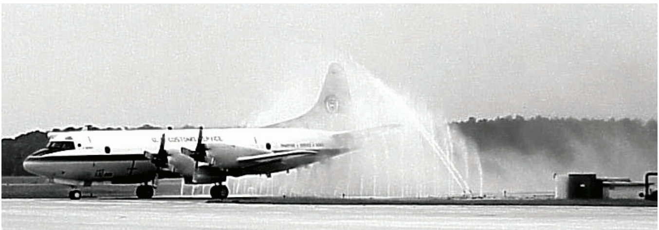
Figure 2-7. Aircraft at a Taxi-Through Rinse Facility
