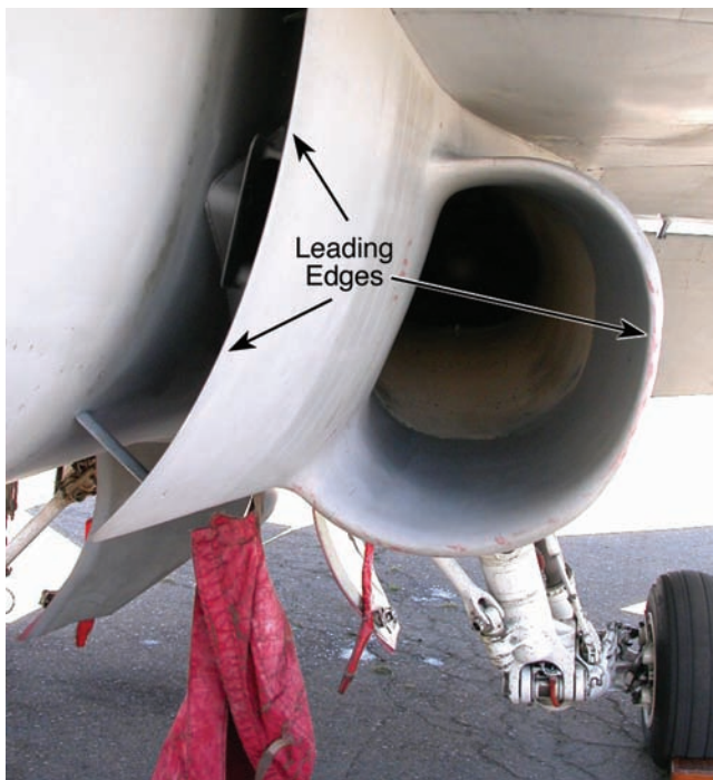
Figure 3-10. Corrosion Prone Points of Air and Engine Inlet
