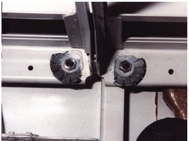
Figure 6-5. EMI Bonding Washers in Avionics Bay
