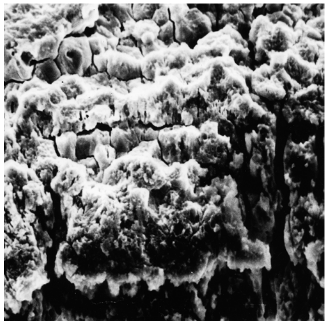
Figure 3-12. Scanning Electron Micrograph of a Corroding Aluminum Surface
