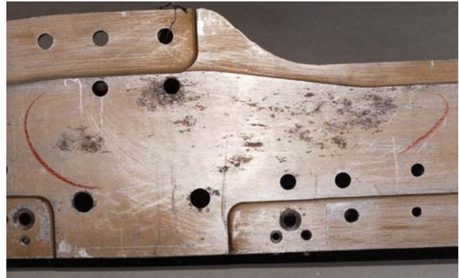
Figure 3-10. Pitting of an Aluminum Wing Assembly
