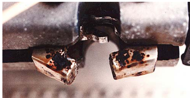
Figure 3-28. Failed Chromium Plate
