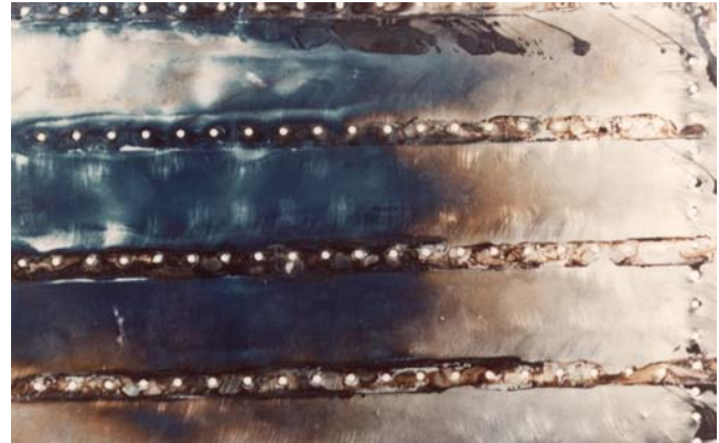
Figure 3-26. Color Changes in Titanium Due to Heating
