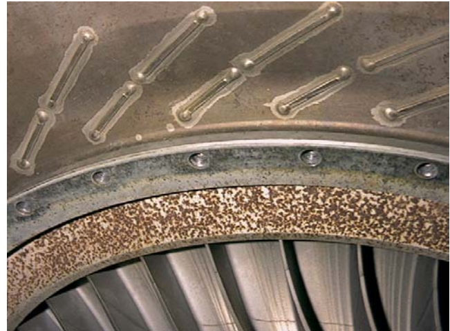
Figure 3-22. Hot Corrosion on Engine Components
