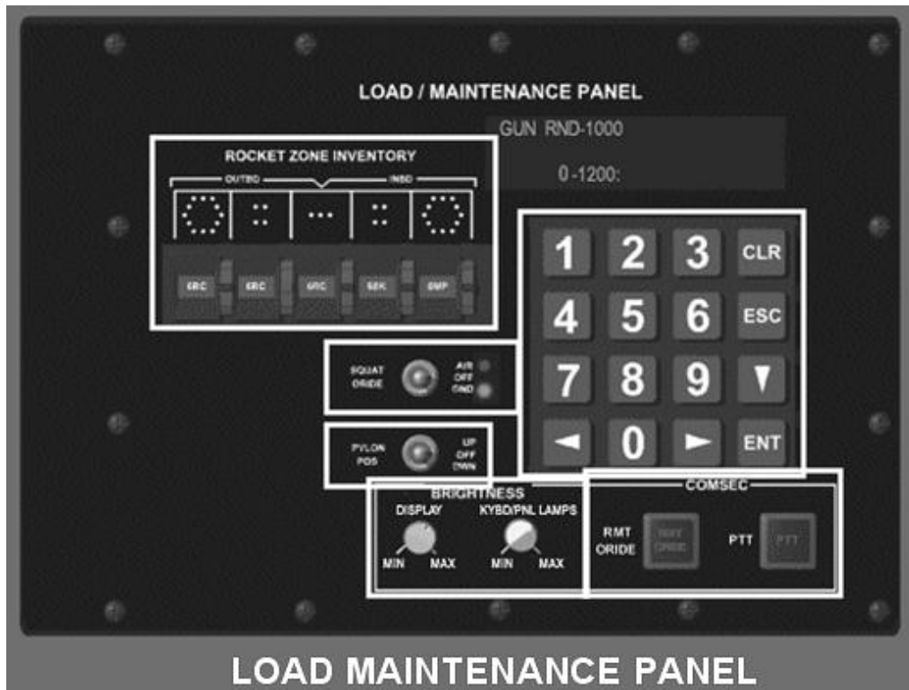
Figure 72. Load Maintenance Panel Layout.
