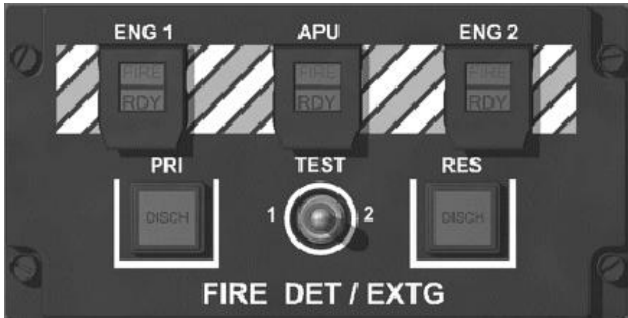
Figure 24. FIRE DET/EXTG Panels.
