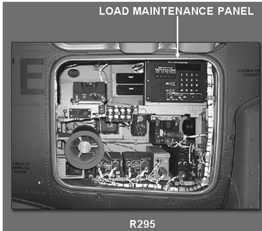
Figure 70. Load Maintenance Panel.
