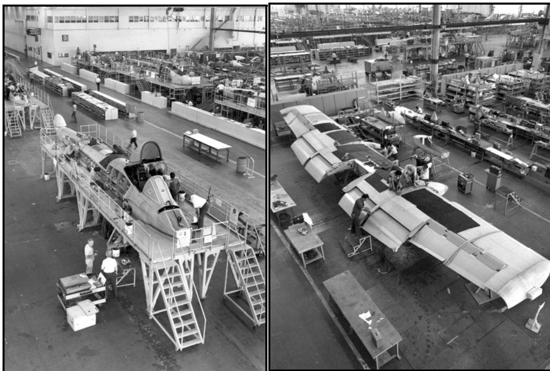
Figure 19. A-10 Fuselage and Wing Production
